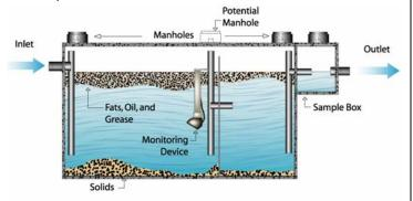
A grease interceptor should be checked and maintained to ensure that it is working properly. Backups, odors, and drainage problems are signs that the grease interceptor is not functioning as it should. See OC San's Fact Sheet for Grease Interceptor for specific tips on proper maintenance of grease interceptors.
